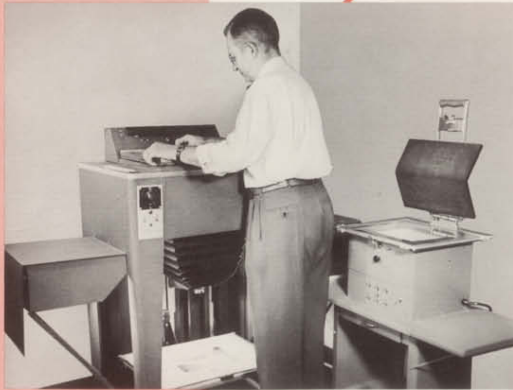
Modern vertical camera used in our Art Department to quickly reduce or enlarge pictures and type for layouts and final art work.
