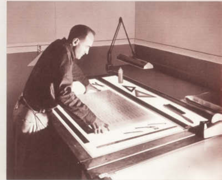
The strip-up department where negatives are carefully examined and precisely stripped up into forms for making plates.
